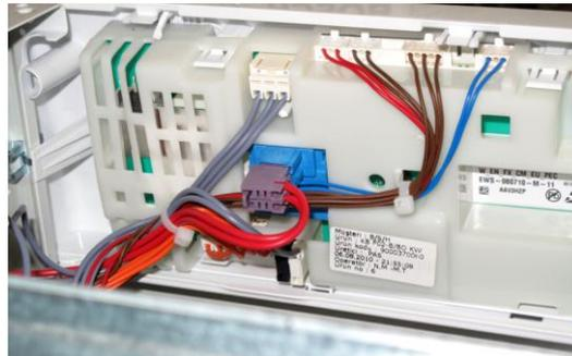
**Figure 3** Siemens front panel wiring and cable routing clips
