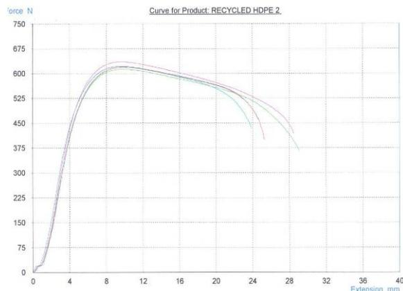
**Figure 3.** Stress/Strain Curves for Recycled HDPE samples
