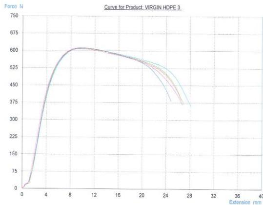
**Figure 2.** Stress/Strain Curves for Virgin HDPE samples
