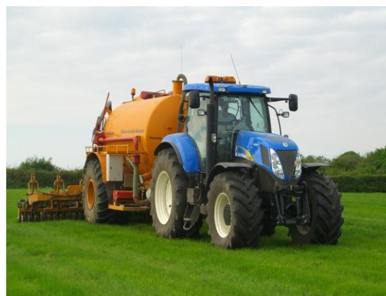
Plate 2. Shallow injection application to grassland
