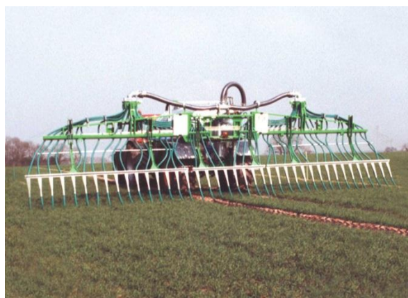
Plate 1. Bandspread application to arable land
