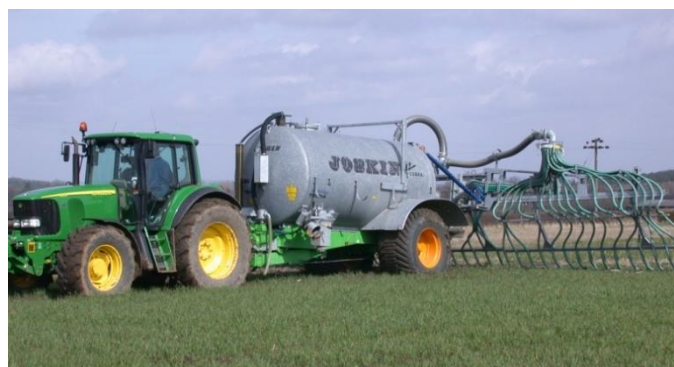
Photo 1: Precision band spreading application of digestate
