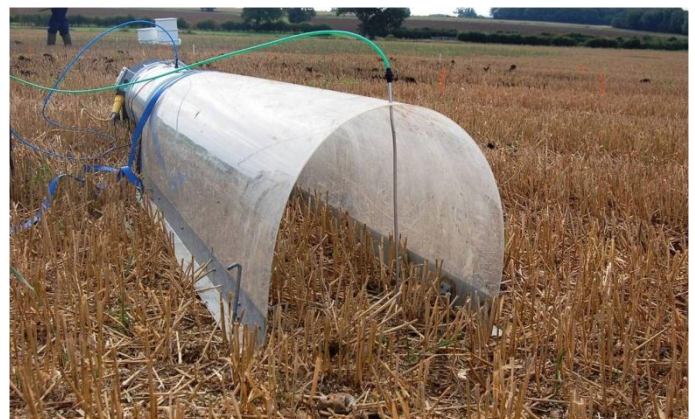
Photo 3: Ammonia wind tunnels measurements at Wensum Nitrogen Hub – autumn 2011
